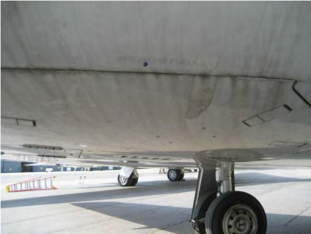
The right wing has evidence of a fuel leak and a hydraulic leak
