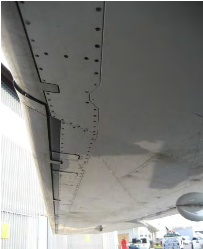
The right wing has evidence of a fuel leak and a hydraulic leak
